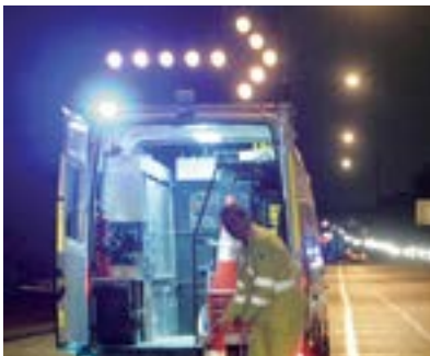
A temporary arrow on a roadwork vehicle warns you that a road hazard is ahead. Change lanes.
