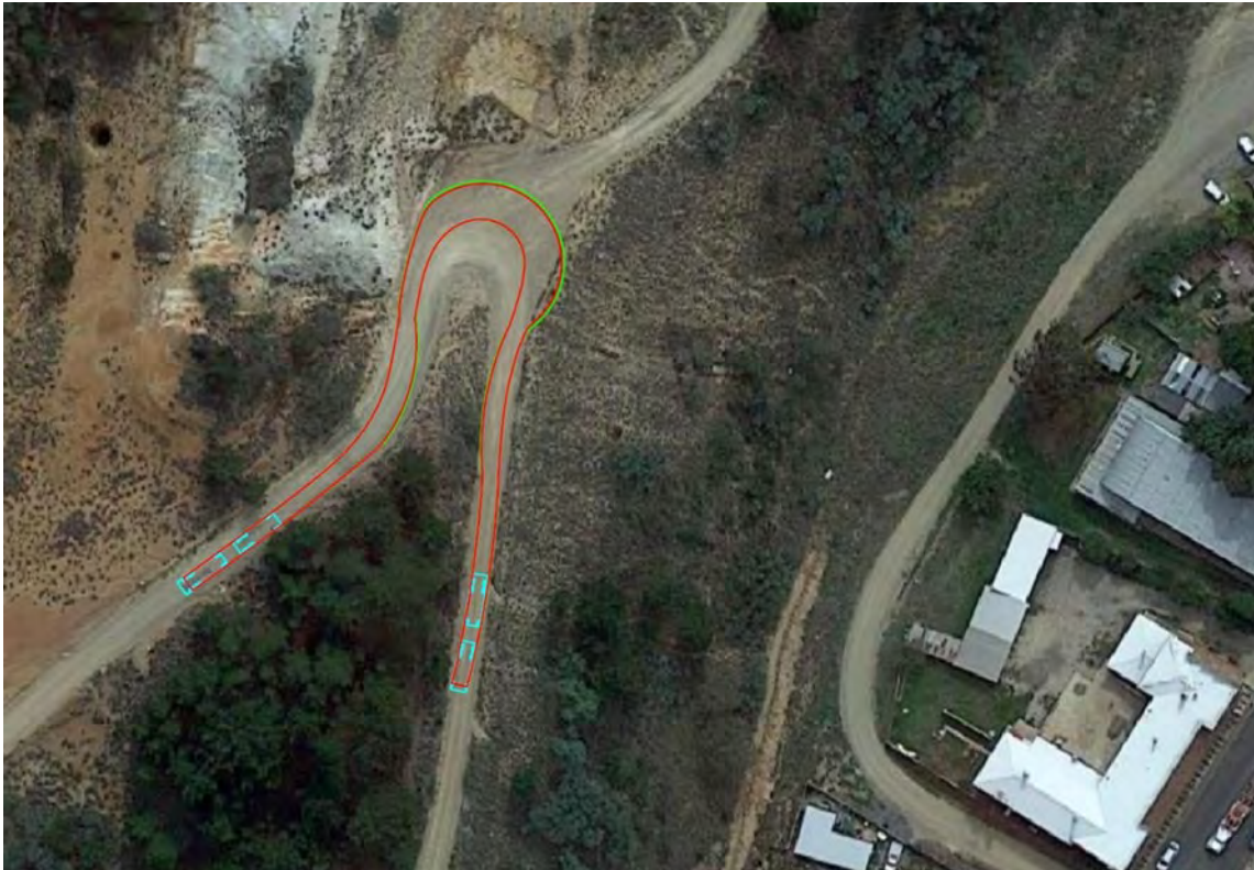
Figure 7-3: Swept path analysis - Miners Road hairpin turn (right) at 5km/hr (truck and dog combination)
