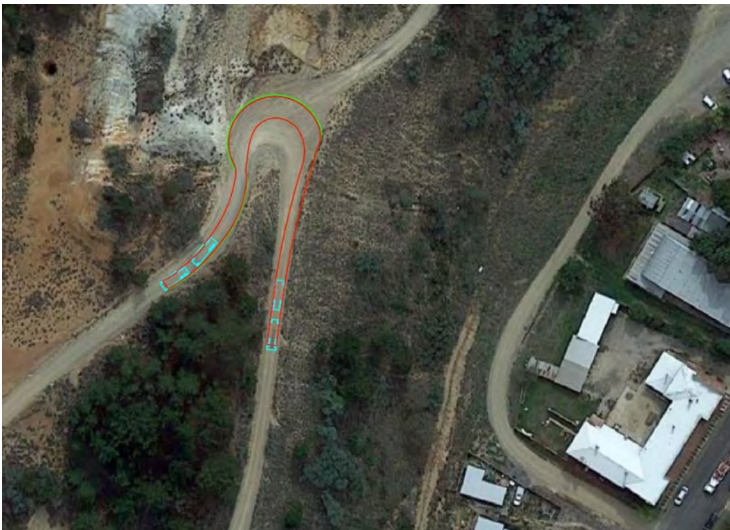
Figure 7-2: Swept path analysis - Miners Road hairpin turn (left) at 5km/hr (truck and dog combination)
